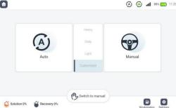
completed, and set the desired cleaning mode and cleaning times. After completing the settings, click the [start Task] button at the bottom right corner of the page. The floor scrubber will carry out the task automatically according to the selected task, the cleaning mode and the cleaning times. Operation steps are as follows:
