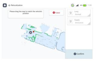
wait until the positioning status in the upper right corner becomes [positioning succeeded], and the green laser line and the edge of the obstacle overlap, which indicates that the positioning is successful. If not, repeat the above operation.
