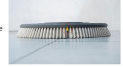
Check whether the strips are damaged, deformed, aged or cracked. If so, please replace them in time.
