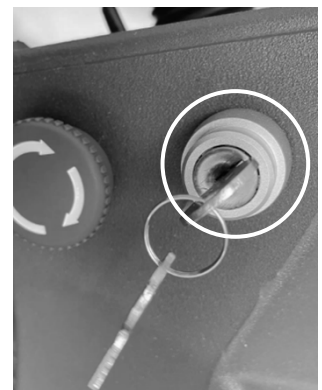
Turn off the power Lift the squeegee and the brush plate.
