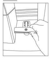
Adjustment of the height of the main brush: use the main brush handle to adjust the position of the main brush.
