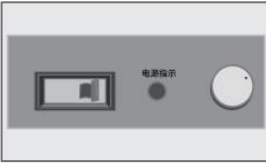
High pressure washing switch Motor speed adjusting knob
